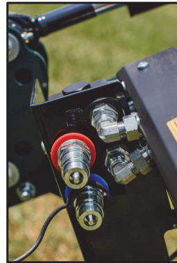
3rd Function Valve Behind Loader Bucket
