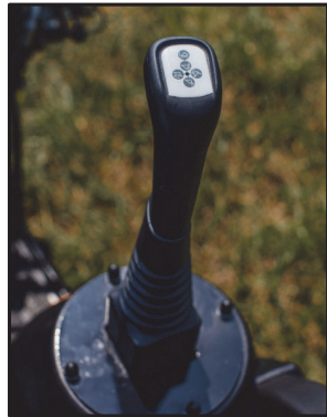
3rd Function Button at Front of Joystick
