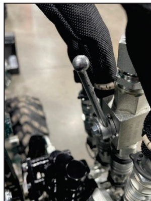
Loader Lower Speed Control Lever
