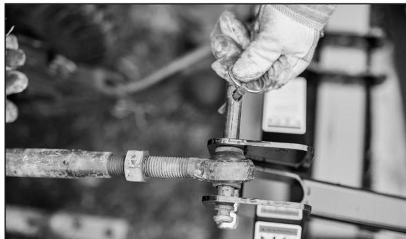
Install center link and mounting hardware.
