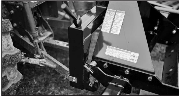
Lower quick hitch hooks.
