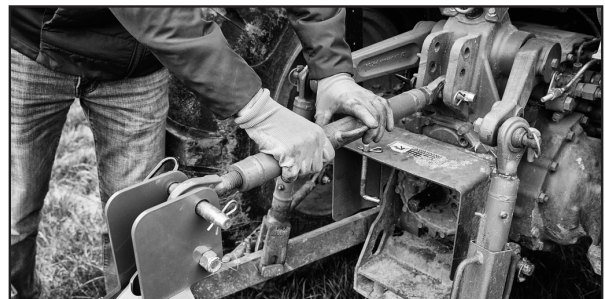
Figure 2: Use tractor top link to tilt front and rear of Land Plane.
