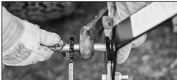
Attach tractor draft link to hitch pin.
