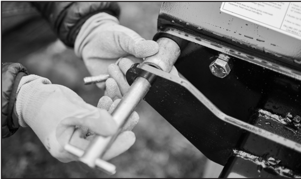
Install bushings before attaching to quick hitch.
