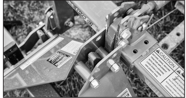
Raise quick hitch and engage hitch pins.
