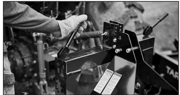
Lower handles to lock quick hitch.
