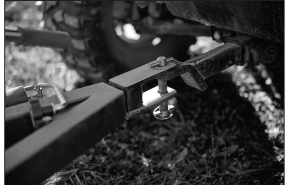
Figure 1 - Connect swivel clevis hitch to power unit and secure with pin.
