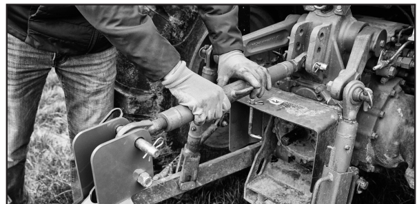
Figure 3: Use tractor top link to tilt front and rear of Box Blade.
